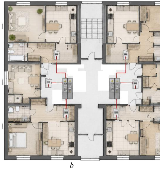
Figure 1 – Power supply diagram for the flats on a floor of a typical 9-storey building
