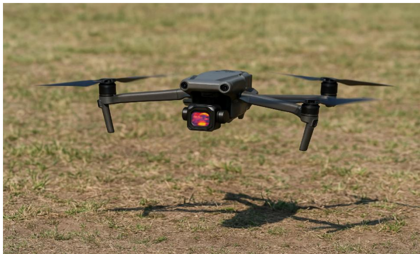
Figure 2. – Drone with Thermal Camera: Drones equipped with thermal cameras can survey large areas to detect landmines based on thermal signatures. (Rzayeva 2025)
