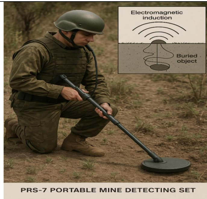
Figure 1. - PRS-7 Portable Mine Detecting Set: Designed for detecting both metallic and non-metallic mines (Daniels, D. J., 2004)
